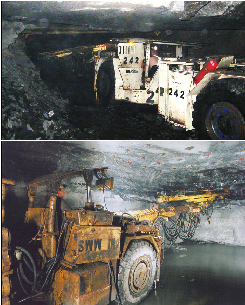
Figure 16.4 Single Boom Drilling Rigs
