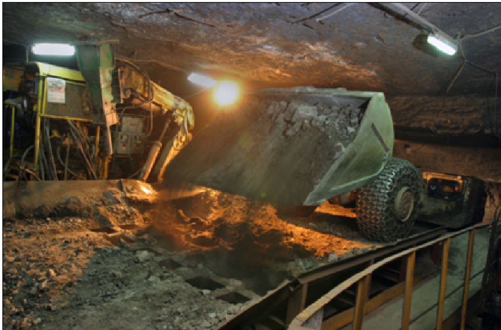
Figure 16.14 Front-End Loader at Rock-Breaker/Feeder to the Conveyor
